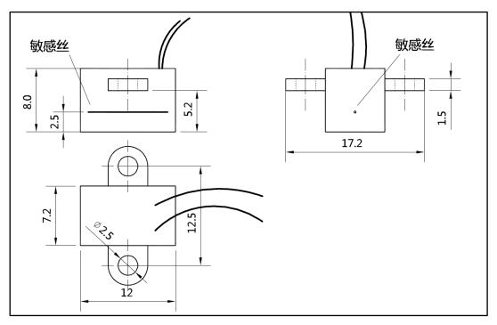
The Pins are soft wire, there is no distinguishing of positive and negative polarity
