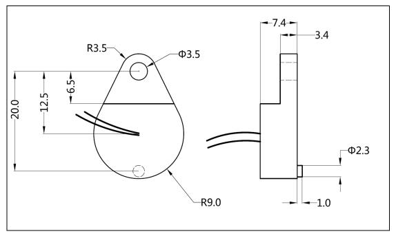
The Pins are soft wire, there is no distinguishing of positive and negative polarity
