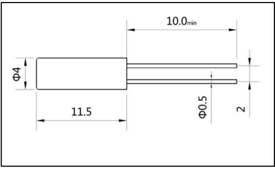
The Pins are tinning copper hard wire, there is no distinguishing of positive and negative polarity
