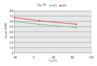
Supply Current (Off) versus Supply Voltage
