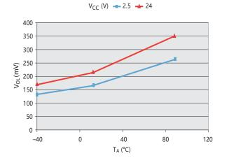
Low-level Output (On) versus Supply Voltage
