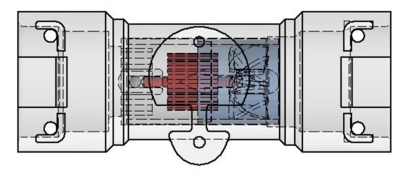
The sensor should be close to the magnetic steel rotor as far as possible, the distance is  $\leq 10$ mm.
